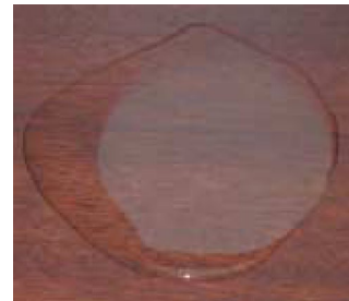
Formation of milky spots caused by water on a freshly coated surface.
