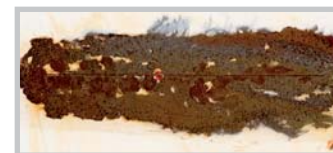
Salt spray test: No rust protection
