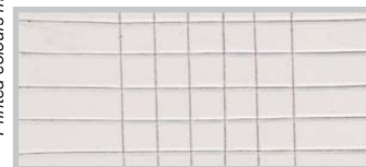
Cross-cut test: Good adhesion
