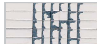
Cross-cut test: Detachment of varnish
