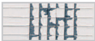
WITHOUT All Primer: The varnish detaches
